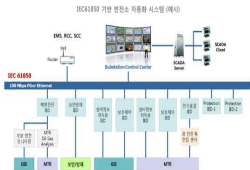
(Figure 2) IEC61850 Based Substation Automation System
