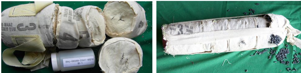
Figure 2. The appearance of broken charge bag
