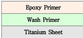
Figure 3. Section shape of specimens
