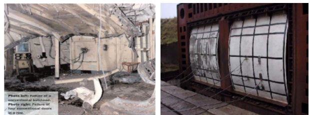
(a) Blast test in a retired ship (b) Validation Test on BHB
