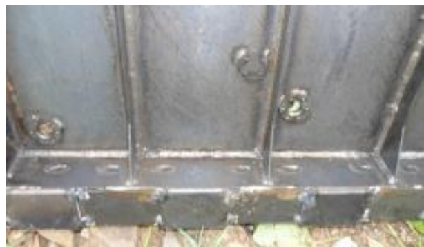
Fig. 4 Spot welding in insert plate with cartridge
