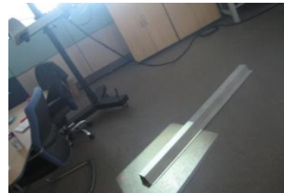
Fig. 4 Measurement of the three-dimensional shape of the side sill with an optical scanner
