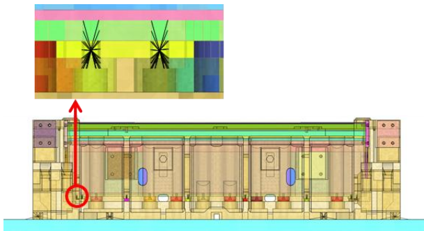
Fig. 9 Boundary conditions for the bolting region and slide contact condition
