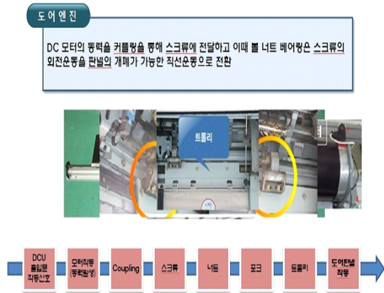
[Figure 2] Operation Process of Electric Door System
