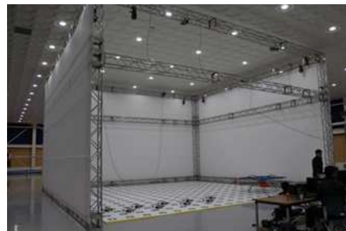
Fig. 5. Motion capture system for the indoor positioning system
