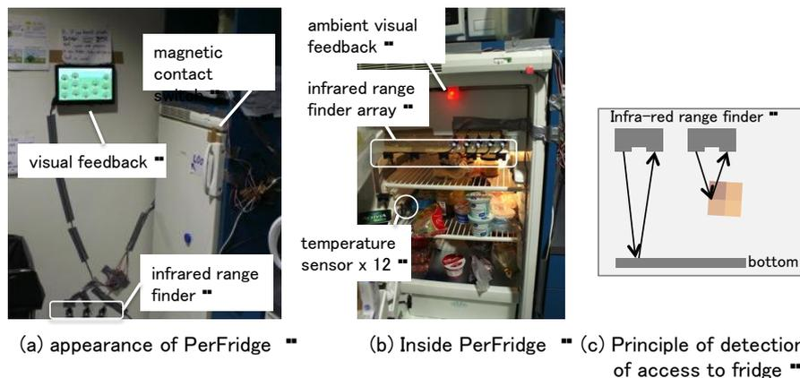
**Figure 2. Installation of PerFridge ((a) and (b)) and the principle of access detection**
