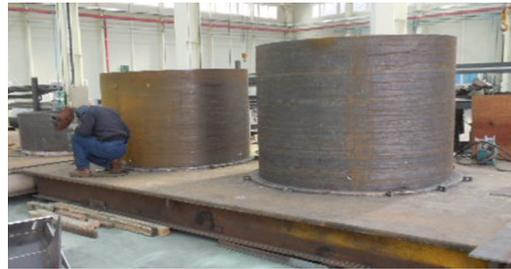
Fig. 2 Bending & welding
