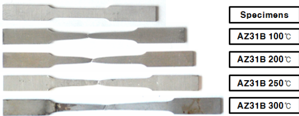
Fig. 3 Specimens of hot tensile test
