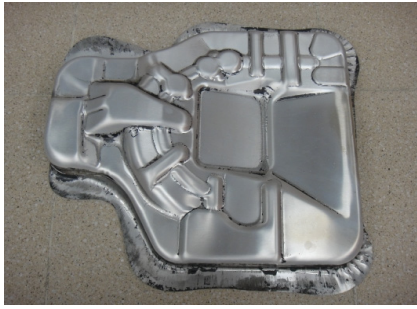
Fig. 18 Drawing product of reinforced dash (thickness: 1 mm)
