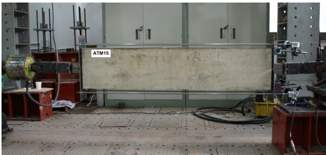
Fig. 4 Direct tension test setup apparatus
