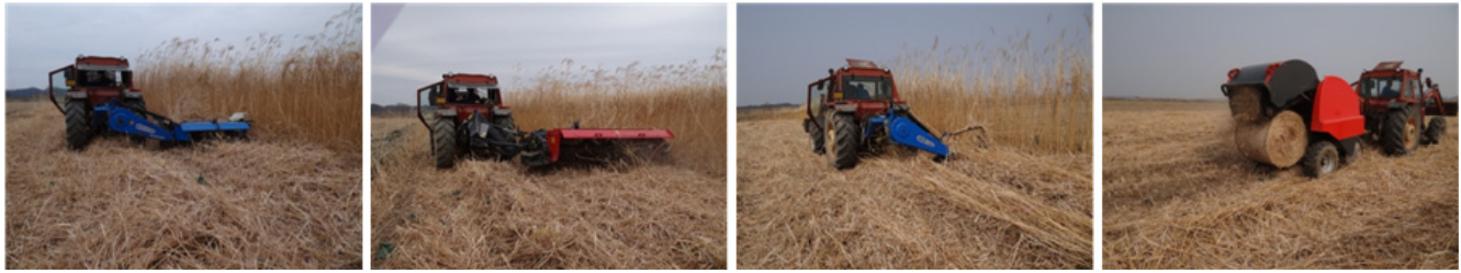
Figure 6. View of operation of different mowing and baling methods to harvest giant miscanthus.
