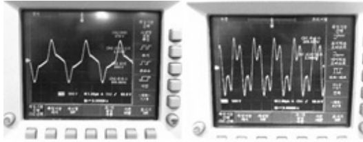
Fig. 5 Output waveform by self resonance according to variable frequencies. (Push-Pull topology, turn ratio 2:80, primary inductance(Lm) 3.3uH, Left:300kHz/ 2kVpeak, Right: 265kHz/ 2.66kVpeak)
