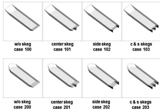
Fig. 18 Top views for attached skeg and without skeg for KNU-001 and KNU-002
