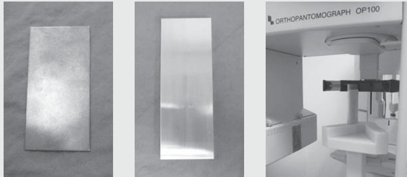
Fig 3. Reproduction of the attenuation of by skull and soft tissue. (Left) 0.8mm copper plate used for reproduction of the attenuation by skull. (Center) 6mm Aluminium plate used for reproduction of attenuation by soft tissue. (Right) The image of attached 0.8mm copper plate to the X-ray source and 6mm aluminium plate in front of test phantom for image taking. (cited from Choi DH, The image quality assurance in digital panoramic radiographs by using the evaluation table and the phantom stand PhD. thesis, Seoul National University 2012.24
