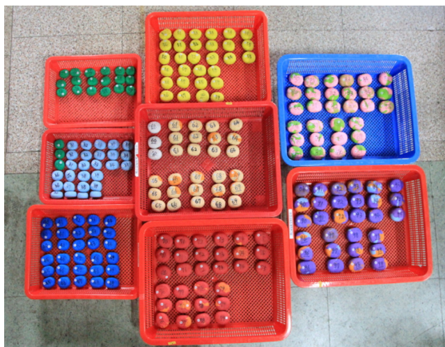
Figure 7. Rubber-clay specimens representative of dry persimmons used in the study.
