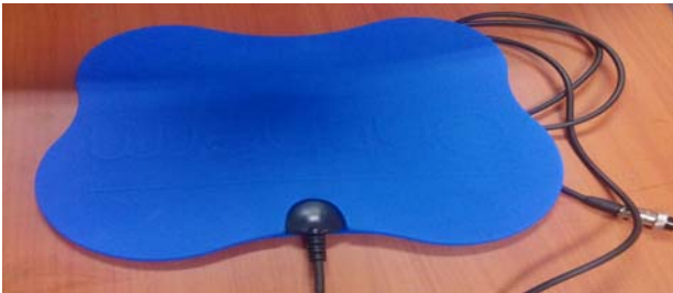
Figure 16: Manufacturing of the insulated earth plate
