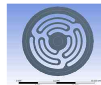
Fig. 3. Sheet spring type check valve
