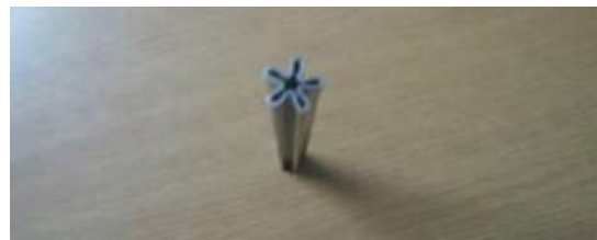
[Fig. 6] Cross section of helical insert device
