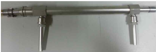
[Fig. 3] Double pipe heat exchanger with helical insert device
