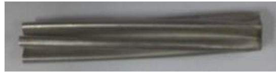
[Fig. 5] Helical insert device
