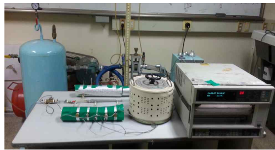
[Fig. 2] Experimental apparatus of double pipe heat exchanger with helical insert device
