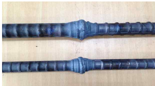
Fig. 12. Specimens with welding joint
