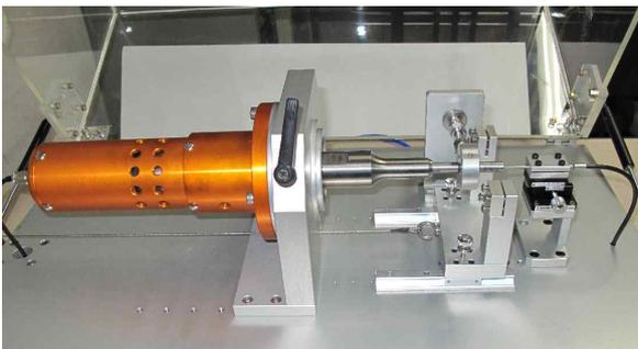
Fig. 1 Ultrasonic fatigue tester
