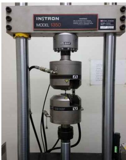
Fig. 2 Hydraulic fatigue tester (Instron 1350)
