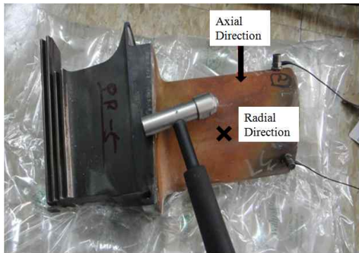
Fig. 3 Measurement of the free frequency
