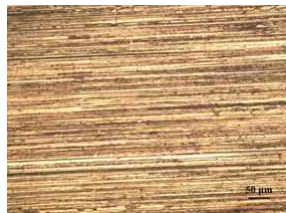
(a) Before treatment including milling lay (STSM)
