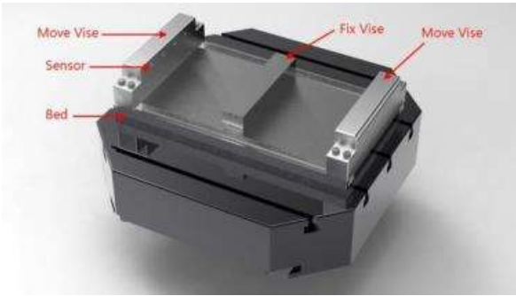
Fig. 4 Pro-E model of clamping unit using zig vise
