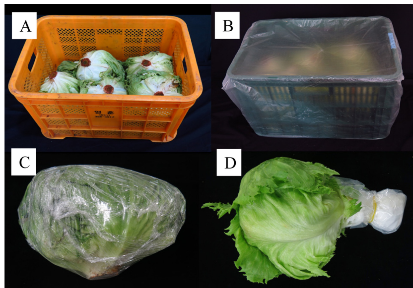
Fig. 1. Four types of packaging used: (A) plastic box container (control); (B) plastic box container covered with high density polyethylene (HDPE) film; (C) plastic box container with lettuce wrapped with linear low-density polyethylene (LLD-PE) film; and (D) lettuce with stem in plastic box container.
