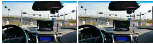
Fig. 8. Example of traffic light recognition.
