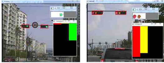
Fig. 7. Example of traffic status recognition.
