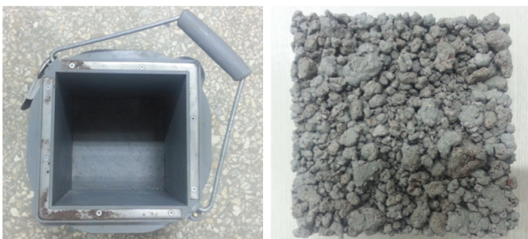
Fig. 2 Fabricating lapilli-cement mixture bio-block (15×15×5cm)
