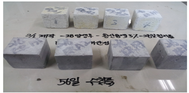
Photo 3 Chemical resistance of polymer-modified mortars
