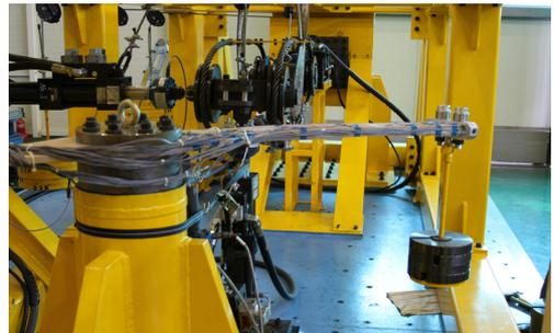
Fig. 3 Flap stiffness measurement of flexbeam
