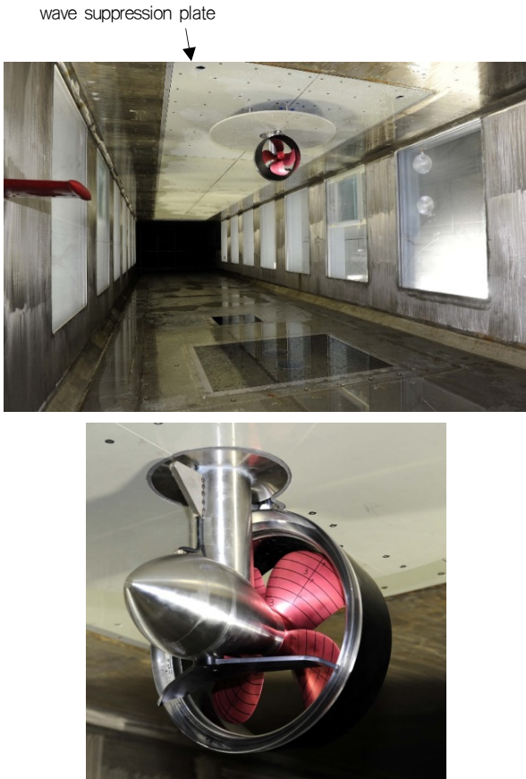
Fig. 9 Photos of the azimuth thruster installed in the test section
