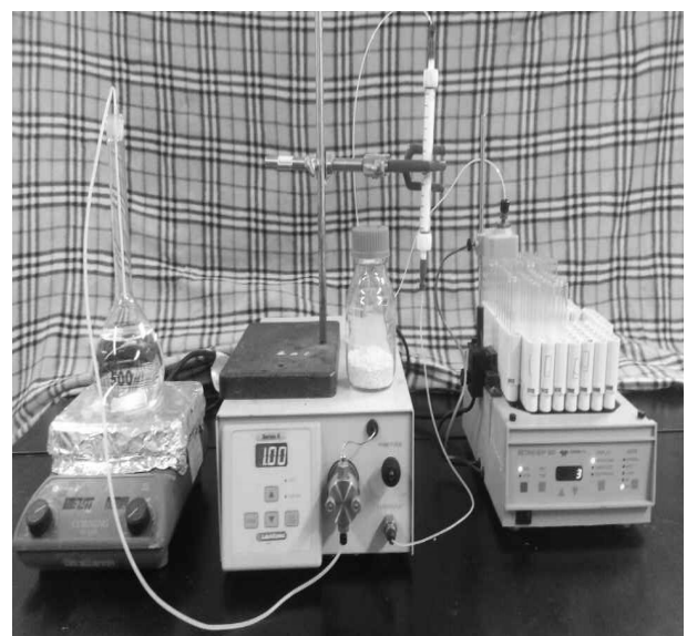
Fig. 1. The apparatus of packed-bed column using Dowex 21K XLT resin
