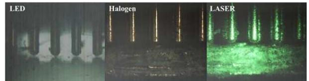
**Fig. 5** Effect of light source types on the acquired image of pin-pad collision observation (LED, Halogen, and Laser source)
