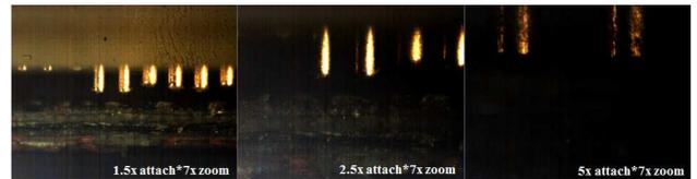
**Fig. 4** Difference of acquired images over various object lenses (Mitutoyo attach lens, 1.5X, 2.5 X, 5.0X at Navistar 7X zoom condition)
