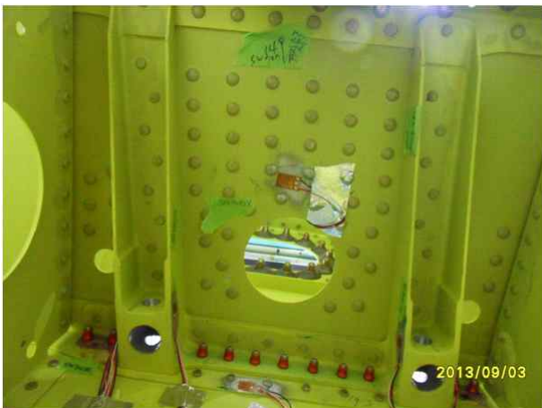
Fig 9 Strain Gages of INBD Pylon Support Structure
