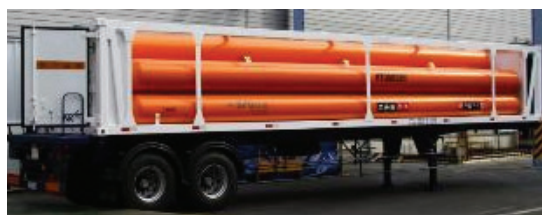
Fig. 1 CNG composite (E-glass/epoxy) pressure vessels loaded on the vehicle
