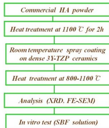
Fig. 1. Experimental procedure of specimen preparation and analysis.
