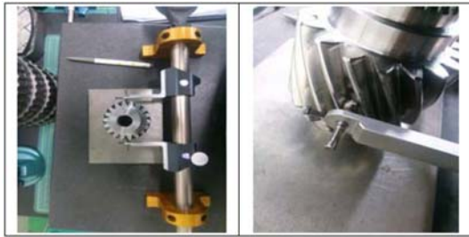
Fig. 4. Strain measurements using the universal gauge.
