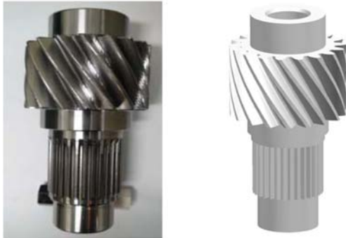
Fig. 1. SCr420HB helical gear shaft.
