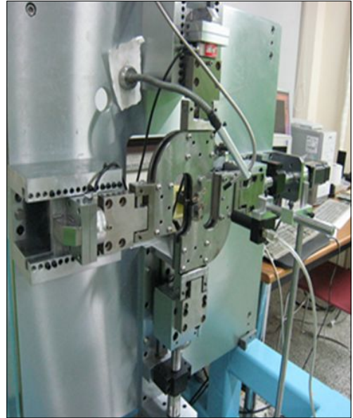
Fig. 3 Schematic diagram of Mixed mode fatigue test system
