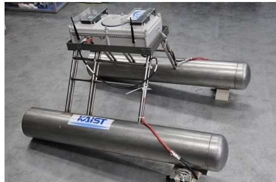
[Fig. 5] JEROS (Jellyfish Elimination RObotic Swarm) developed by KAIST (2012).
