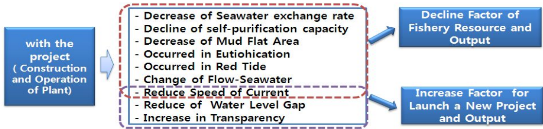
[Fig.2] Marine Environment Influence by Construction of Tidal Power Plant in Garolim Bay
