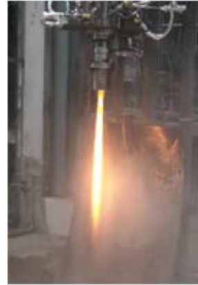
Fig. 4 Combustion test performed by Chungnam National University using hydrogen peroxide and kerosene propellant.
