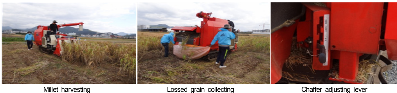
Figure 6. Experimental method for grain loss testing in field using the combine harvester.
