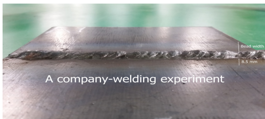
[Fig. 10] The width of welders and welding bead height by company experiments
