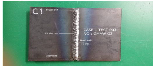
(b) B company weld bead shape
