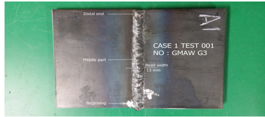
(a) A company weld bead shape
