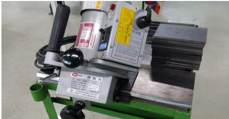
[Fig. 2] Specimen deburring machine
