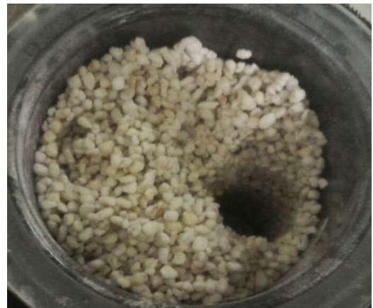
Fig. 5 Reactor bed after hydration using perlite supporting calcium chloride.
