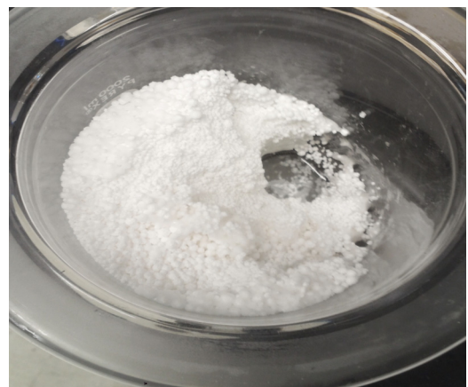
Fig. 4 Reactor bed after hydration using calcium chloride.
