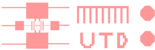
Fig. 2. Test patterns used for the electron beam lithography of high-aspect-ratio nanoscale patterning of SU-8.
