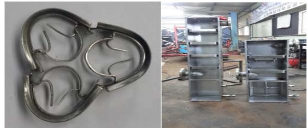
**Figure 2:** Photos of packing and wet scrubbers
