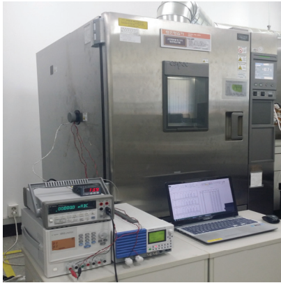
Fig. 4 Picture of the test setup for power loss measurement
