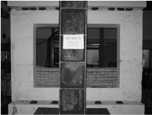
Fig. 14 Test result of PD-SRCF specimen(500gal)
