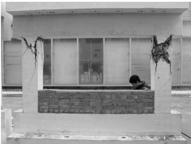
Fig. 11 Test result of PD-RC specimen(300gal)
