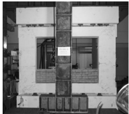
Fig. 13 Test result of PD-SRCF specimen(400gal)
