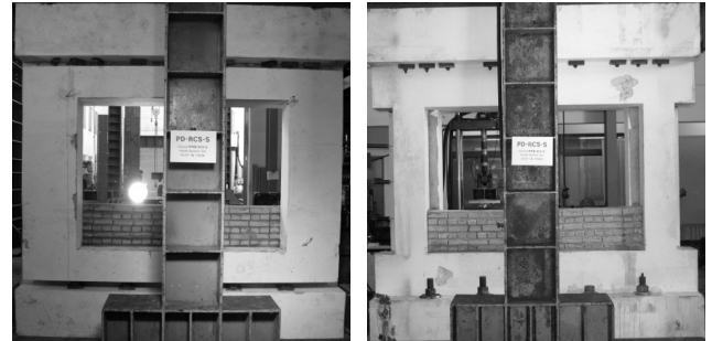
(a) Front view (SRCF strengthening) (b) Rear view (Existing frame)
