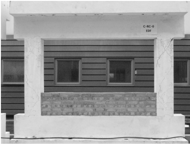
Fig. 10 Test result of C-RC specimen
