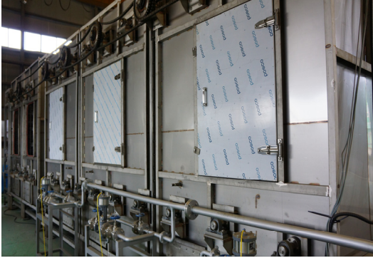
Fig. 9 Experimental apparatus of continuous sterilizer
