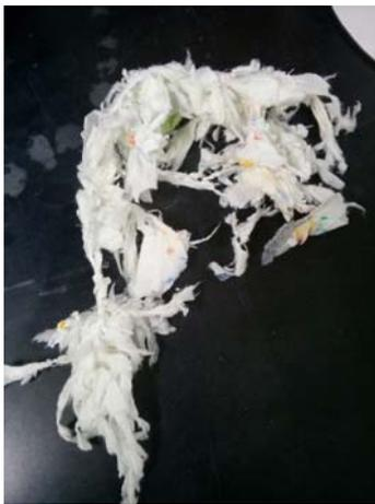
Fig. 4. Plastic rope formed by pulping action.
